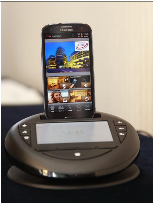
GCC is not only a multiple charging station, but also an IP speakerphone and can be the room Internet access point.
